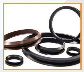
V-rings are rubber face seals. The V-ring is mounted on the shaft and seals the counter surface. A V-ring is produced slightly smaller than the shaft itself, cou sing it to clamp onto the shaft. The lip of the seal prevents liquids and dust from the outside.
